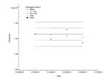
**Figure 1**: FID area response development for the isoprene peak from stored vs. freshly loaded carbon adsorbent cartridges using an isoprene mixing ratio of approximately 25 ppb (500 mL sample size), similar to what is typically found in cartridges taken from seedling leaves in the greenhouse.
